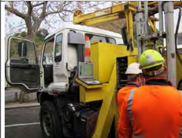
Figure 21. GEOTECH CPT rig, computer real time recording
