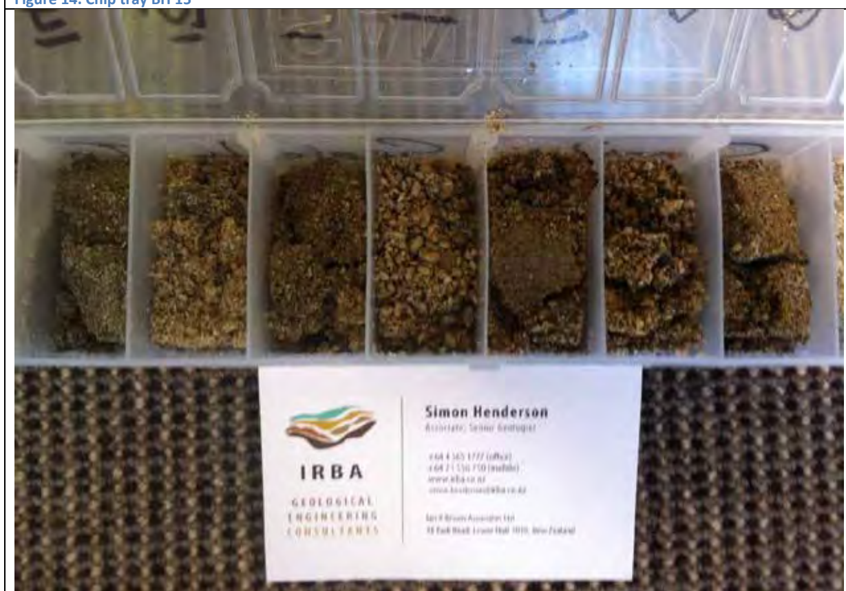
Figure 15. Chip tray close up BH 15 8-15m
