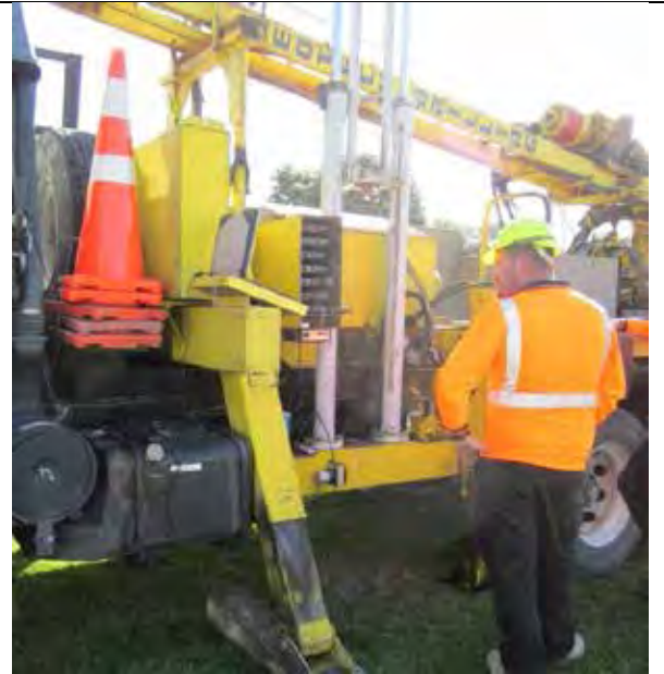
Figure 20. GEOTECH CPT rig, zero'ing electrics
