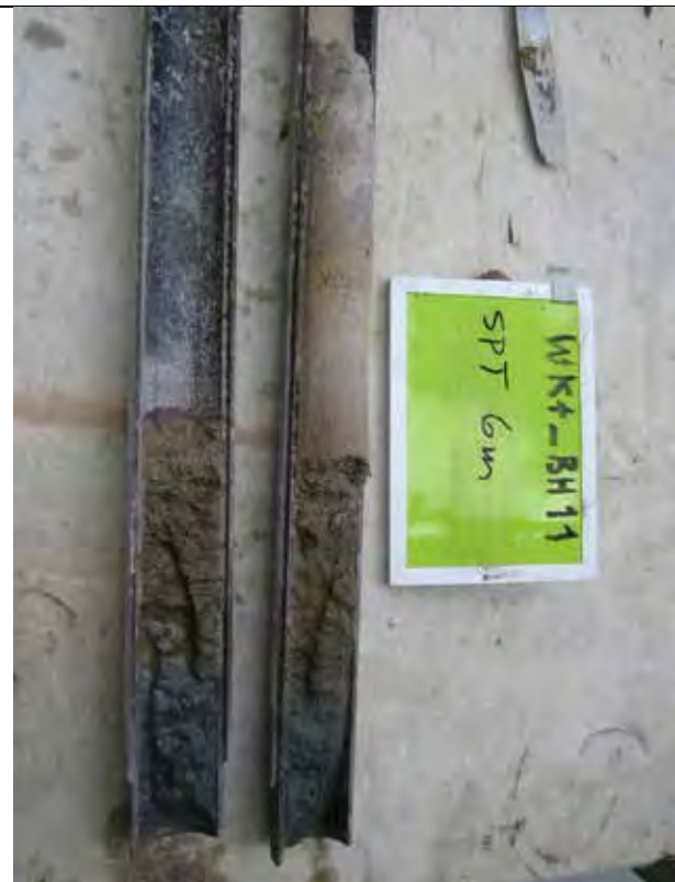
Figure 11 SPT record: WKT BH11 SPT 6m.
