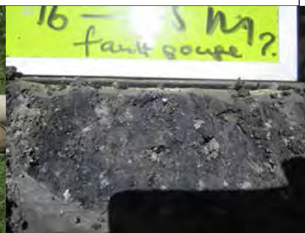
Figure 13. Close-up photo: WKT BH11 splits 16m fault gouge?
