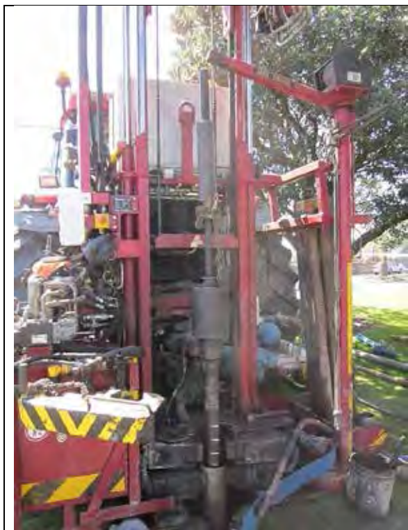
Figure 8. SPT hammer in progress
