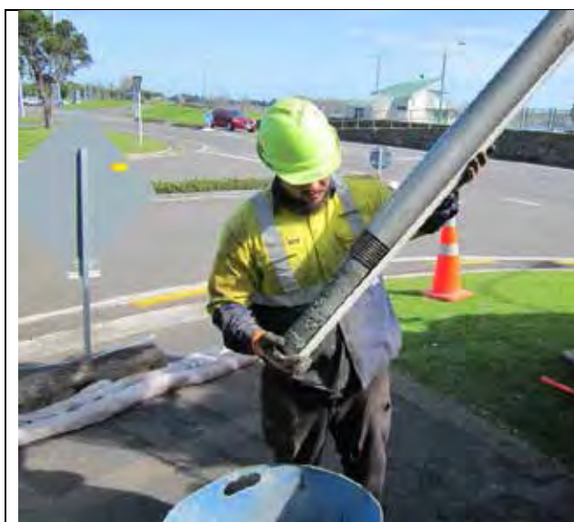
Figure 6. Sonic split sample extrusion
