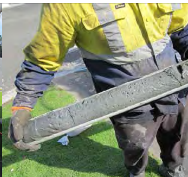
Figure 7. Sonic split tube sample complete
