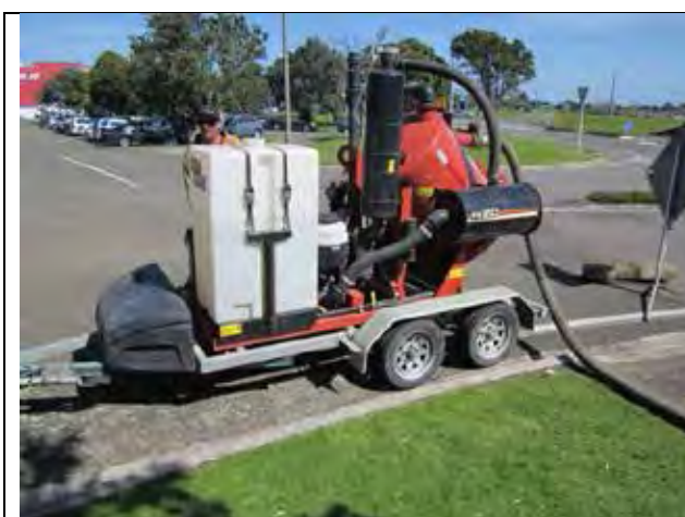
Figure 23. GEOTECH Vacuum trailer
